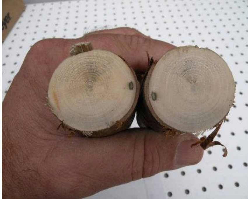
Figure 13. Cross section of failed red maple branch. Wood-staining fungi have colonized the area of crushed cells on the lower portion of the branch, discoloring the area of compression failure. The area of torn fibers is also evident in the upper portion of the branch.
