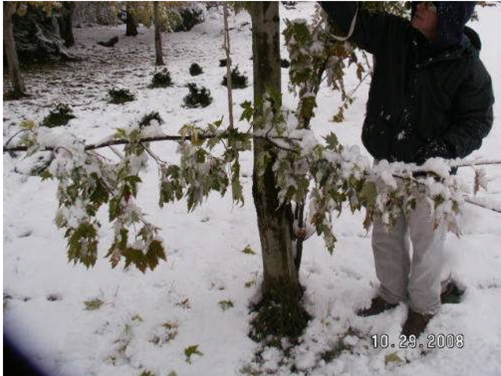
Figure 36. Weighing a small silver maple branch heavily loaded with snow. The branch being weighed is suspended horizontally from the tree from which it was removed.
