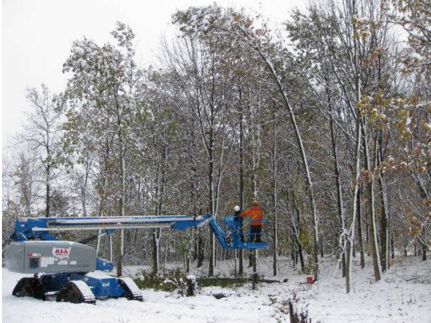
Figure 37. Assessment of the effect of crown reduction pruning on snow loading. Changes in stem deflection were recorded as the tree was pruned.
