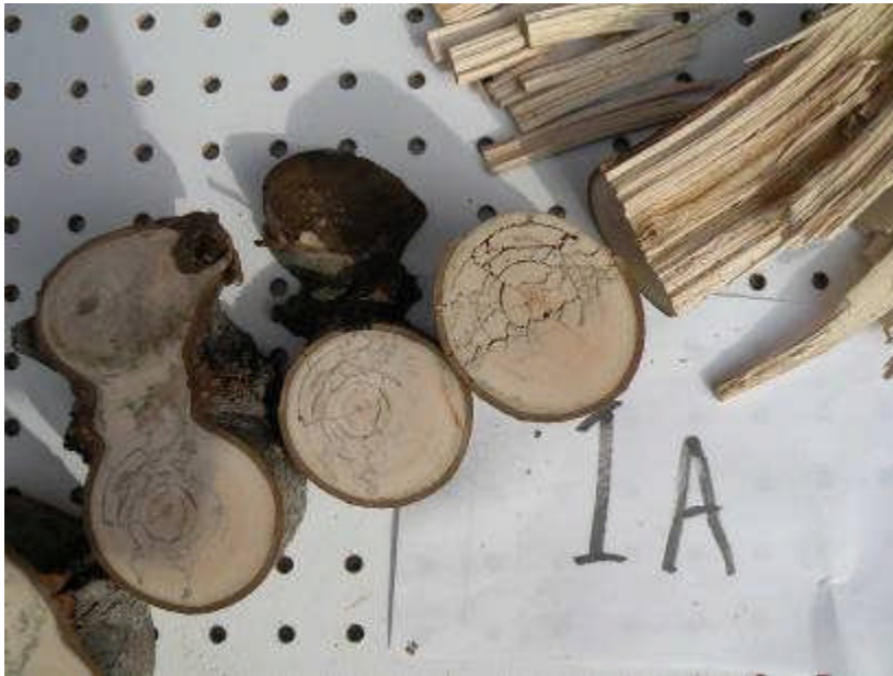
Figure 10. Examples of stem dissection in the failure zone. Evidence of fracture can be seen as wood fibers were torn in the upper portion of the branch's cross-section.
