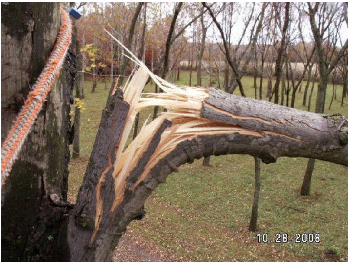
Figure 11. A failed silver maple branch following static load test. Note the compression bands on the underside of the branch, and the torn wood fibers on the upper surface in the fracture zone.
