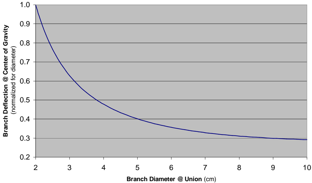
Figure 20. Projected change in branch elasticity based on application of mechanical engineering principles. Results adjusted for changes in branch mass with diameter, and changing length of lever arm.
