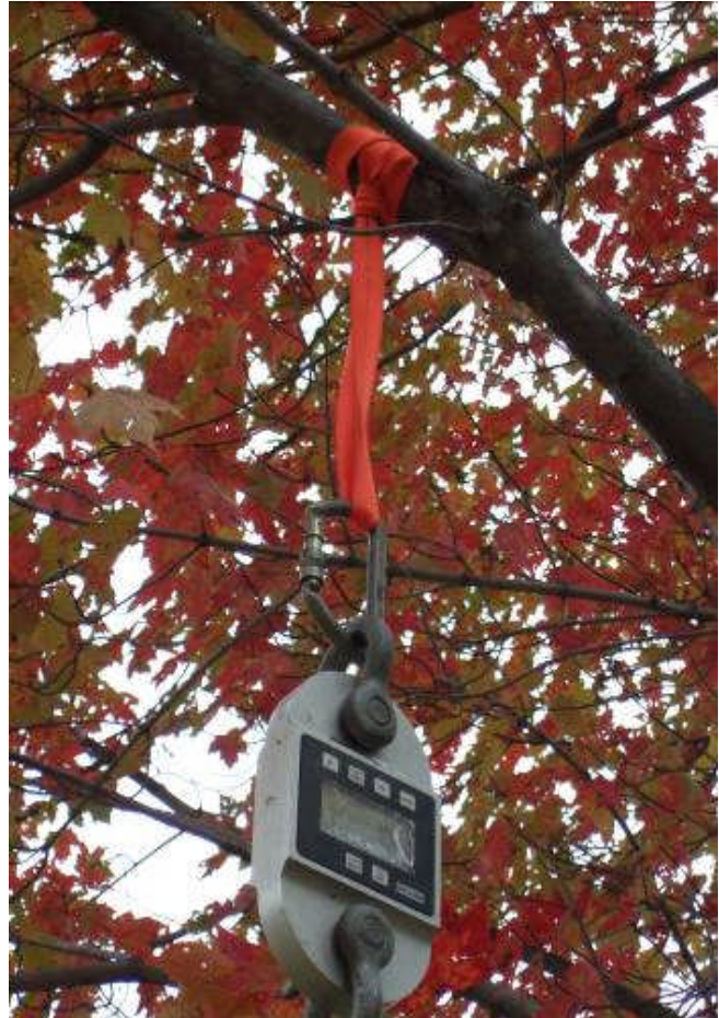
Figure 9. Pulling bridle and load cell in place on test branch.
