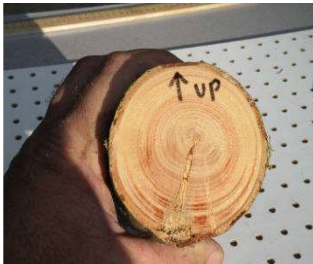
Figure 14. Cross section of failed Eastern white pine branch showing compression crack on the underside of the failed branch section.
