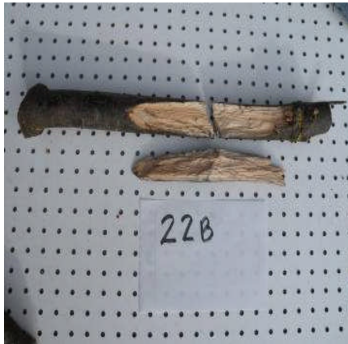
Figure 15. Underside of failed Eastern white pine branch with compression wedge evident.
